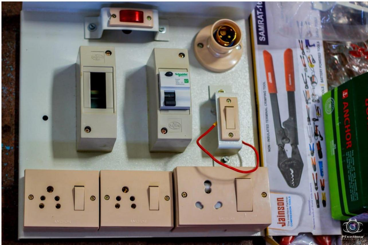
*Photo: Low-cost electric distribution board*
