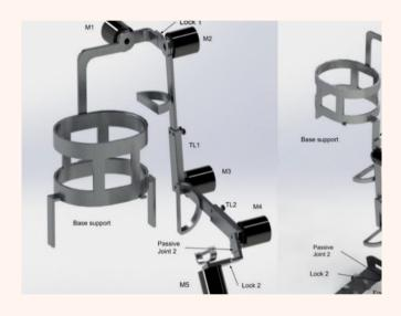
The exoskeleton is designed such that it can be used for both upper limbs and lower limbs, interchangeably.
