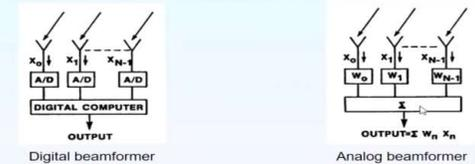
**Digital beamforming:** N number of signals from N antennas passes through analog-to-digital converters. Direct signal processing from computer.
