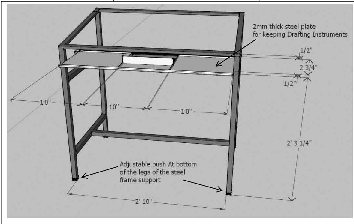
Figure 4. Front side view of Steel frame
