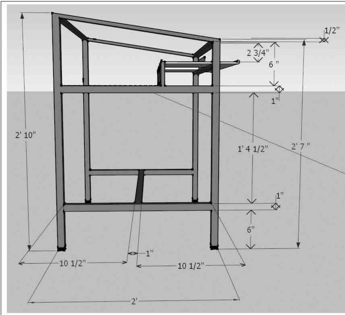
Figure 3. Left side view of Steel frame
