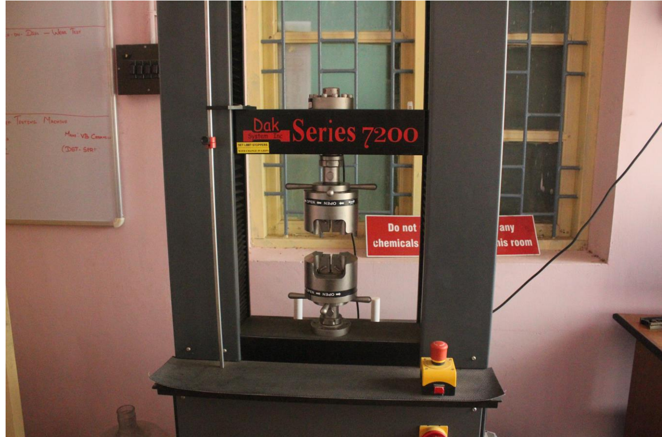
Micro Tensile / compression Instrument (Cold/ hot / Cryo atmosphere)
