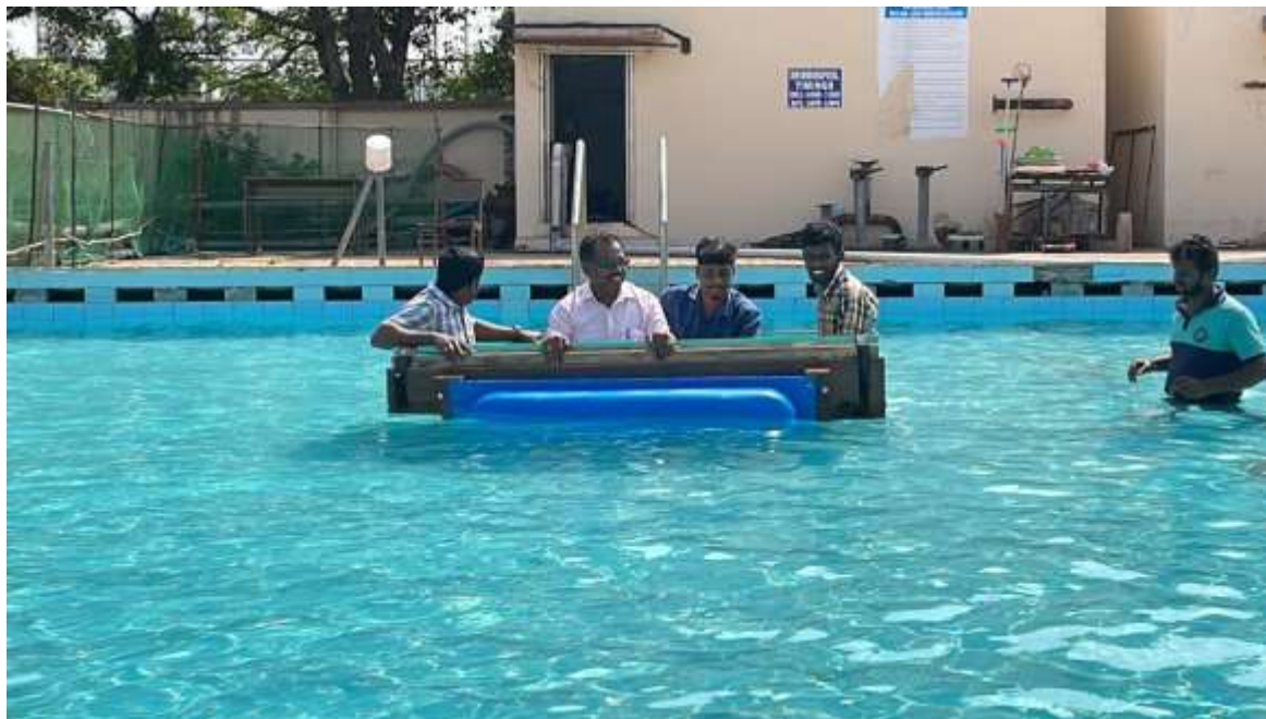
Fig. 6 a,b,c and d Improved design which can be used as furniture, cot and almerha in normal time and can be used as a emergency boat in case of flood
