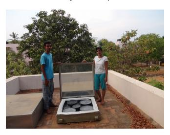
We have made some changes to it apart from the yearly renewal of the black paint for the collector plate and vessels. Initially we used cotton cloth and rubber beading to achieve the seal between the glass plate and the wooden frame. The cotton cloth got charred very fast and the rubber deteriorated fast with use. So, we changed the seal to fibre-glass tape and fibre-glass sleeves. These could withstand the high temperatures inside the solar cooker.
