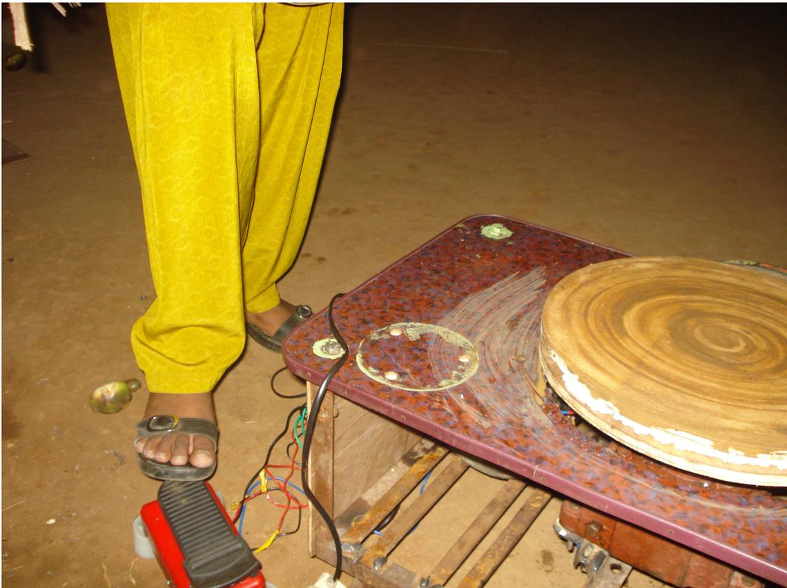
**A foot-pedal for speed control of the potter's wheel frees both hands for pot making**
