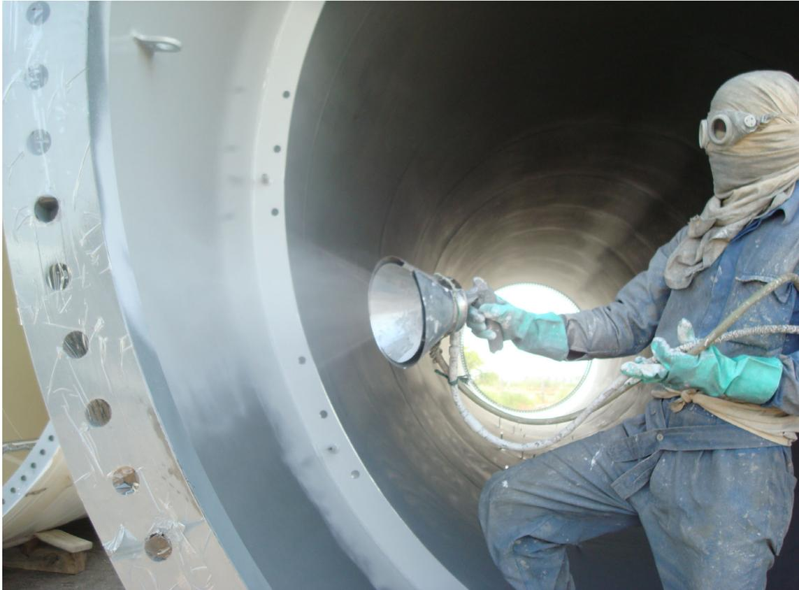
**The paint spray is confined to a cone by the air curtain around it.**
