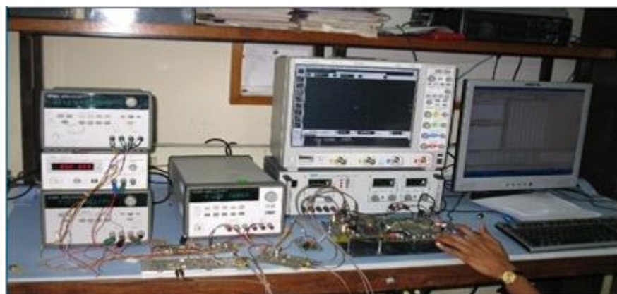
Fig. 5 Integration of RF front end boards with Digital backend board including ADC & DAC boards.
