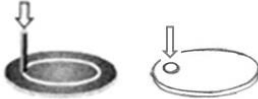
Figure 1. Pin-on disc and ball-on disc set-up.
