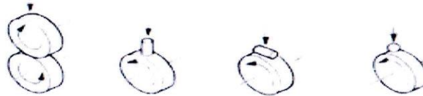
Figure 1. Test configurations of roller-on-roller, roller-on-pin and roller-on-ball.
