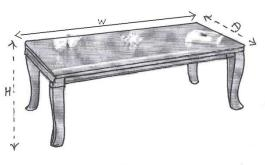
Width (W) = 1200 mm Depth (D) = 600 mm Height (H) = 450 mm
