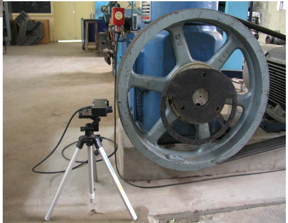
Instantaneous swept volume measuring arrangement
